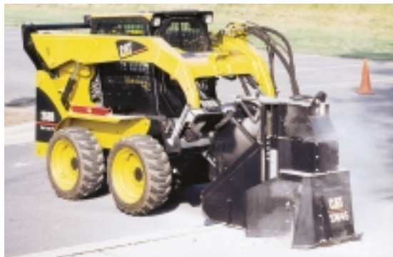
The new Caterpillar 268B skid-steer loader features the high-flow XPS hydraulic system. A variable-displacement piston pump provides hydraulic flow and pressure up to 33 gal/min (125 L/min) and 4060 psi (280 bar) when running high-flow work tools.
