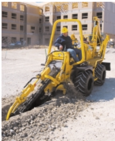
The Vermeer RT450 hydrostatic riding trencher/plow is powered by a 50-hp (37-kW) Deutz F3L2011 engine.
