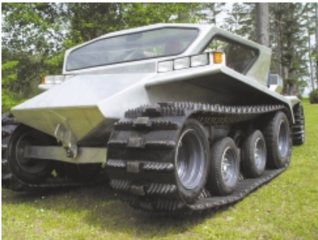
The Iguana prototype vehicle is designed to operate in combinations of deep snow, mud, sand, swamp, and hard surfaces of ice, rock or pavement. The center blocks on the track support the vehicle on paved roads, while the cone-shaped grousers provide traction without damage over soft ground.
