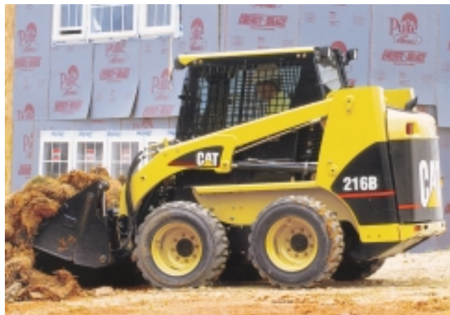
The 216B, the smallest in the new line of skid-steer loaders from Caterpillar, retains the 3024C engine that produces 49 hp (37 kW), and has a rated operating capacity of 1400 lb (635 kg).
